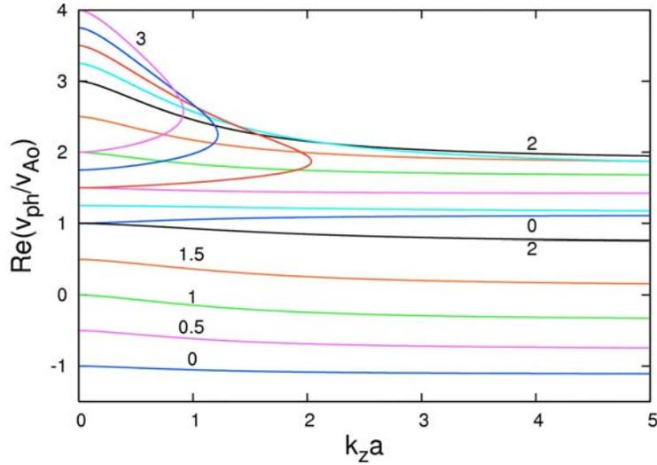
Fig. 9: Dispersion curves of forward and backward propagating conventional sausage waves for different values of the relative Alfvénic Mach number  $M_A$ .
