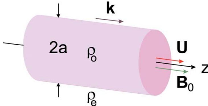
Fig. 1: Geometry of a solar wind flux tube containing flowing plasma.
