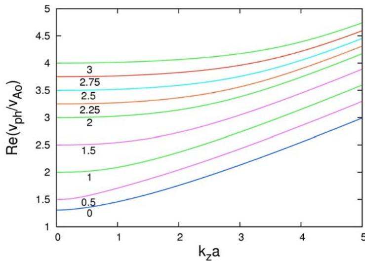
Fig. 6: Dispersion curves of the fast forward propagating Hall-MHD kink waves for different values of  $M_A$ .
