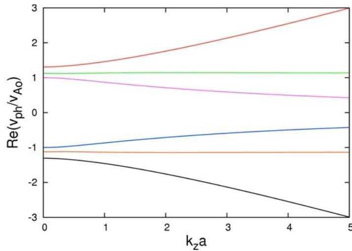
Fig. 5: Dispersion curves of forward and backward propagating Hall-MHD kink waves for  $M_A = 0$ .
