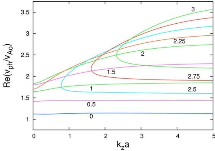
Fig. 7: Dispersion curves of the Alfvénic forward propagating Hall-MHD kink waves for different values of  $M_A$ .
