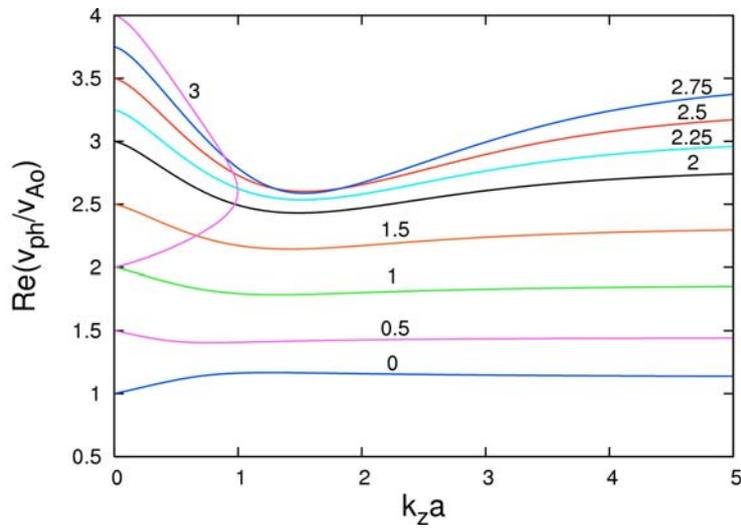
Fig. 13: Dispersion curves of the Alfvénic forward propagating Hall-MHD sausage waves for different values of  $M_A$ .
