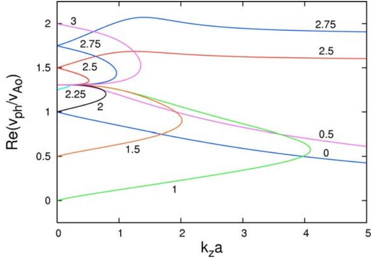
Fig. 14: Dispersion curves of the sub-Alfvénic forward propagating Hall-MHD sausage waves for different values of  $M_A$ .
